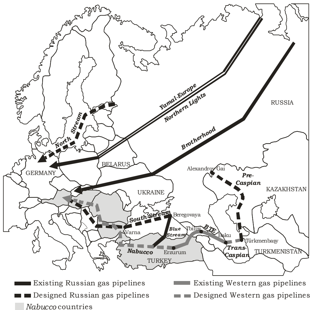
Fig. 2. Map of existent and designed gas pipelines in the Eurasian region
